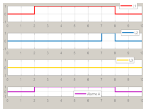
Figure 21: LED States and Alarm
