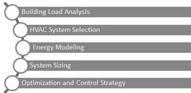
Figure 1: HVAC System Design Process for NZEBs
