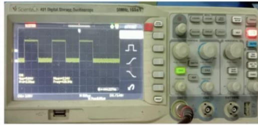
Figure 4.4: Inverter Gate pulse
