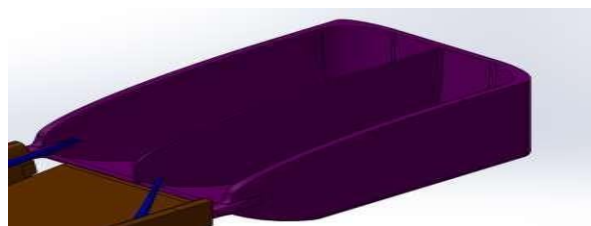
Figure 17: Carriage Design to Collect the Pollutants
